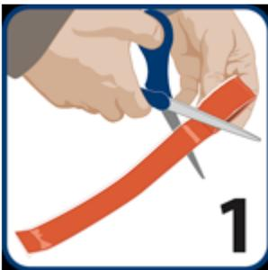
Clean the surface that will be wrapped and cut off the length of tape to be used.
