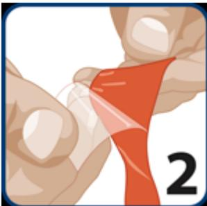
Remove and discard the clear separation film. Heat Tape works on either side.
