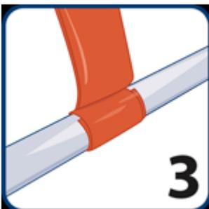
Hold one end of the Heat Tape in position against the object to be wrapped and apply a complete wrap around the object and back onto itself. This initial wrap secures the tape for additional wraps.
