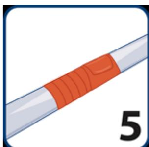
Be certain the end of the final wrap is pressed down onto the prior wraps. Use less stretch on the final wrap.
