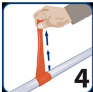
Maintain a constant stretch as you continue to wrap, making sure each new layer “half laps” onto the previous layer. These overlaps will fuse together.
